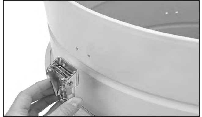
Figure 24. Installing drum latches on collector drum.
